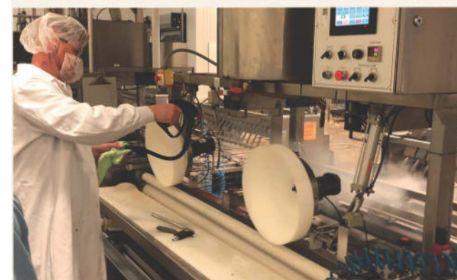
Steam tenting for complete lethal temperature contact
