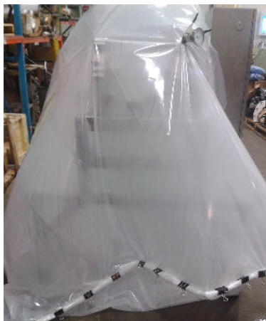
Steam tenting for complete lethal temperature contact
